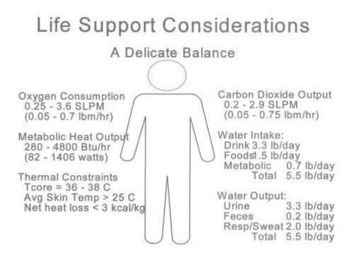
Notes: SLPM – standard liters per minute SLPM – standard liters per minute Figure 1 – Submarine Material Balance
